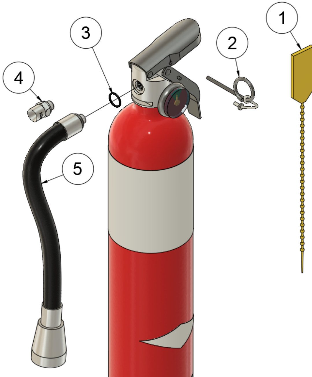
Figure 1. 375H673 & 375N69953 Fire Extinguisher Assembly
